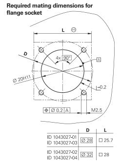
At least 4 mm of load-bearing thread length.
