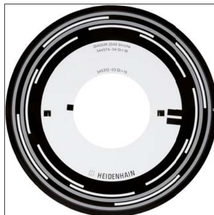
Circular scale with block commutation tracks
