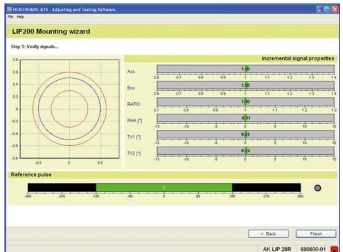
Commissioning using PWM 20 and ATS software
